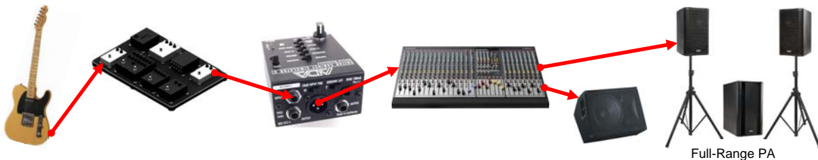
Diagram 1: Guitar to pedal board to GCS-5 to console to monitor speakers and house speakers – no stage amp
