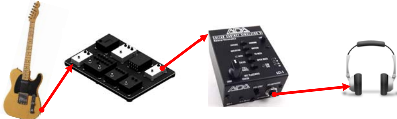
Diagram 3: Guitar to pedal board to GCS-5 to your headphones.
