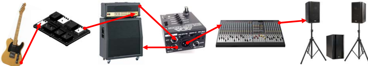
Diagram 2: Guitar to pedal board to GCS-5 split via the THRU jack to your stage amp and the processed signal to the house sound system
