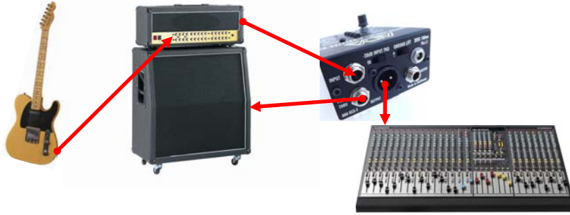
Diagram 4: Guitar to pedal board to GCS-3 to the recording or PA console.
