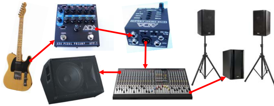
Diagram 6: guitar to GCS-3 to GCS-3 to headphone mix and to studio monitors.
