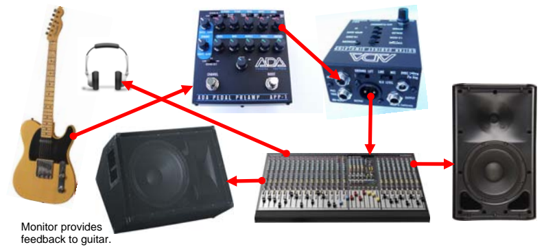
Diagram 6: guitar to APP-1 to GCS-2 to headphone mix and to studio monitors.
