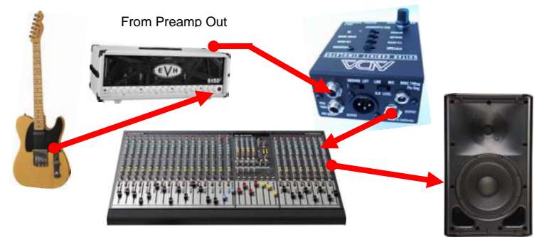
Diagram 5: Guitar to amp head to GCS-2 to sound reinforcement system – no stage amps.
