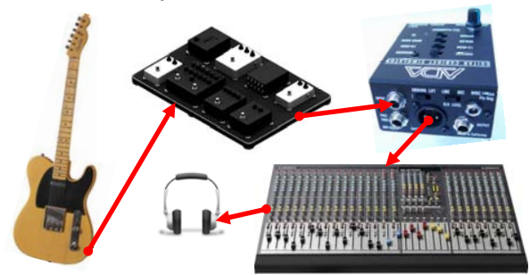
Diagram 4: Guitar to pedal board to GCS-2 to the recording console and to your headphone mix.
