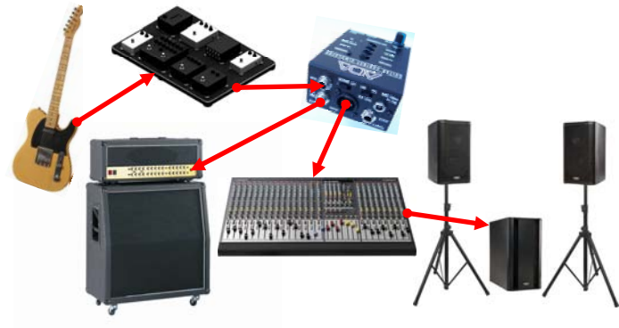
Diagram 2: Guitar to pedal board to GCS-2 split via the THRU jack to your stage amp and the processed signal to the house sound system
